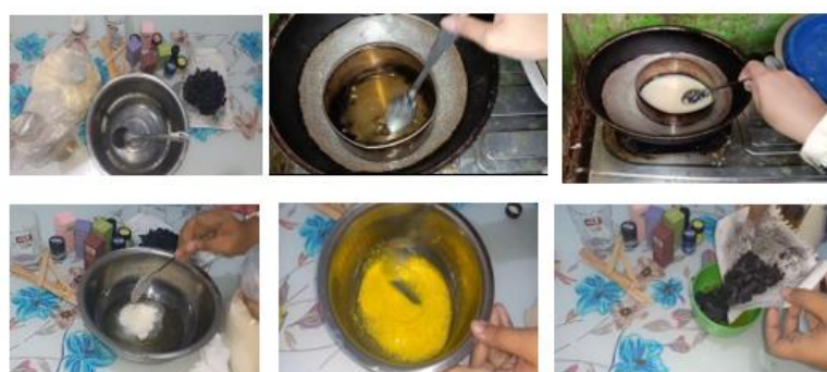
Figure 1. Production Process of Aromatherapy Candles from Waste Cooking Oil
