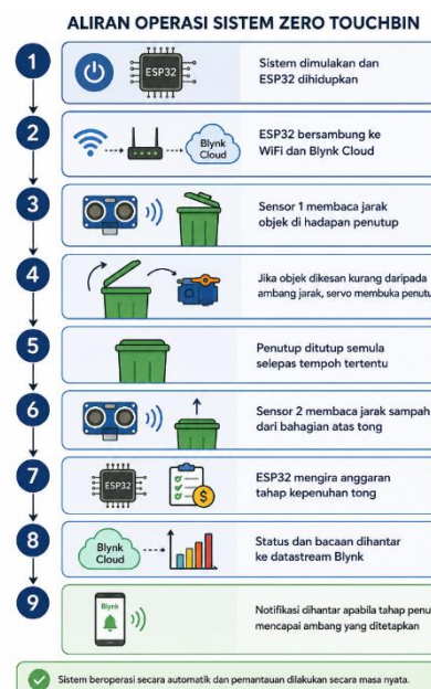
Figure 1. ZeroTouchBin system operation flow
